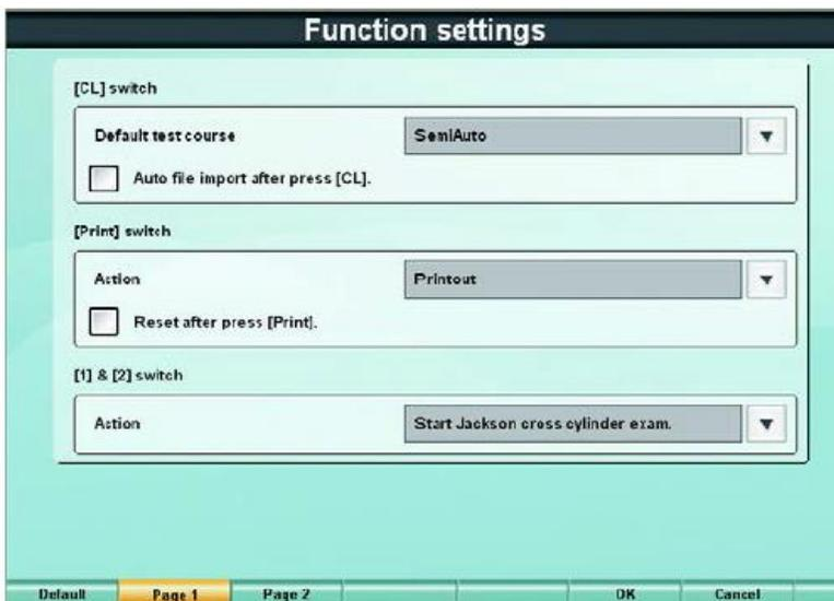
Change [Print] Switch function from Printout to: Output Data or Output Data and Print.
